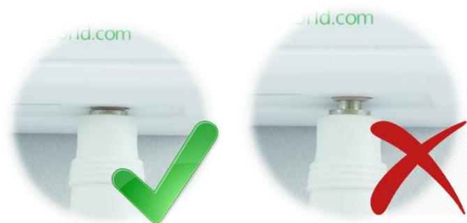
**NOTE!** Check that the sensor is inserted all the way into the 3.5mm red jack socket right to the very end. You must ensure that there is no gap between the connector of the sensor and the jack socket. **Do NOT apply excessive force! – This will damage the jack! If insertion of the sensor feels stiff, gently ease it in rotating it clockwise then counter clockwise.**
